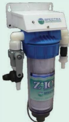
The Z-Ion uses bimetallic ions to disinfect your entire watermaker, including the filters and membranes. It prevents bacteria growth for up to a month and eliminates the "pickling process." The Z-Ion is completely automatic and energy efficient, drawing only 15 watts during the fresh water flush cycle and less than one watt in stand-by. All Spectra Watermakers are retrofittable for the Z-Ion.
